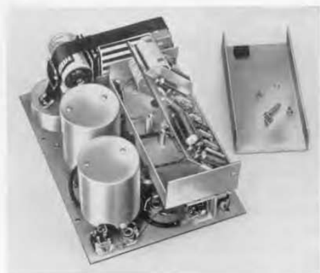
Figure 3. View of Type 1551-A removed from its case. Amplifier cover removed, and amplifier raised to show accessibility.
